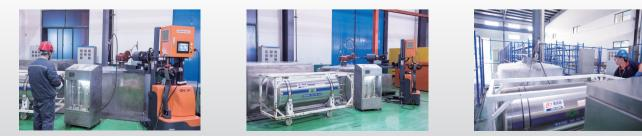
The company has a full set of cryogenic valve test equipment, including full-size liquid nitrogen pool, valve seat leakage flowmeter, torque and test machine, helium detector, to provide capability and product research and development and production test.
